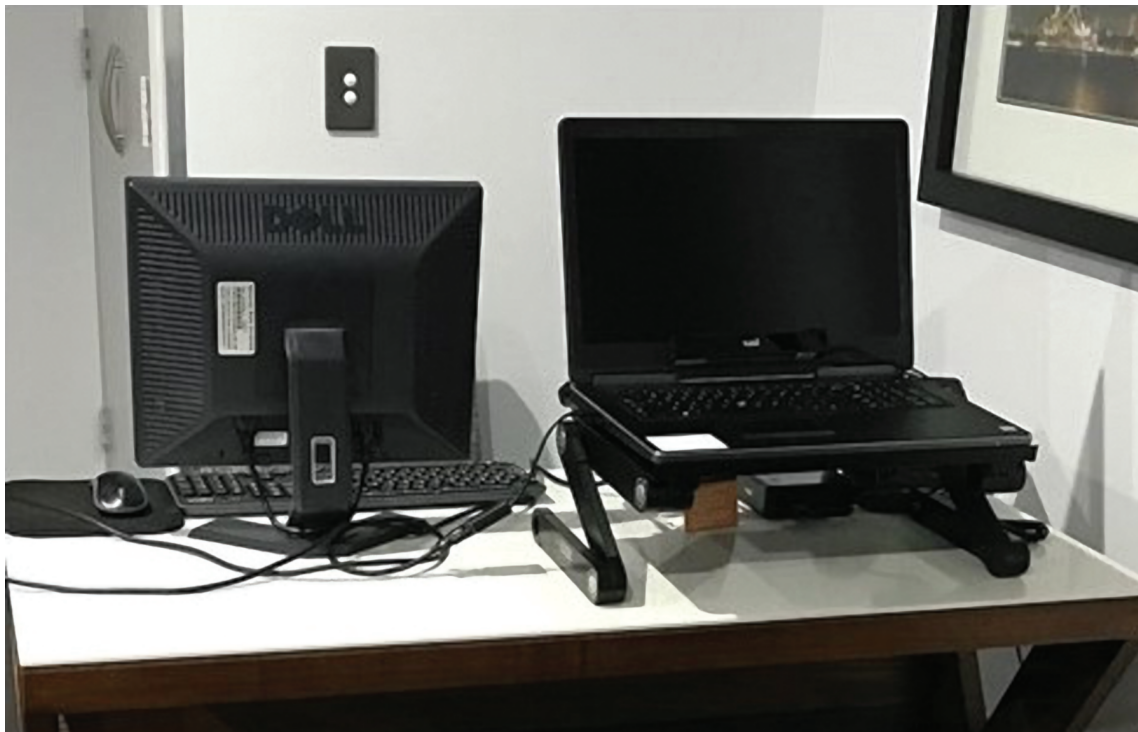
Figure 4. The eye-tracking computer, pictured at the right, rests on an adjustable laptop stand. The experimenter controlled all activities and recorded all verbal responses by keyboard and mouse from the operator station, pictured on the left. This ensured that the participant’s gaze remained on the eye-tracker screen during the gaze recording sessions.
